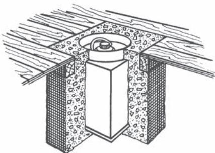
When properly installed in concrete, STAR® Floor Safes provide excellent fire and burglary protection. Now, with the water resistant dust cover, you get protection from water as well.
