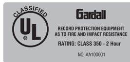
One-Hour exposure to severe fire with an exterior temperature to 1700°F, and an interior temperature that does not exceed 350°F (paper chars at 405°F) for one hour and cool down.
